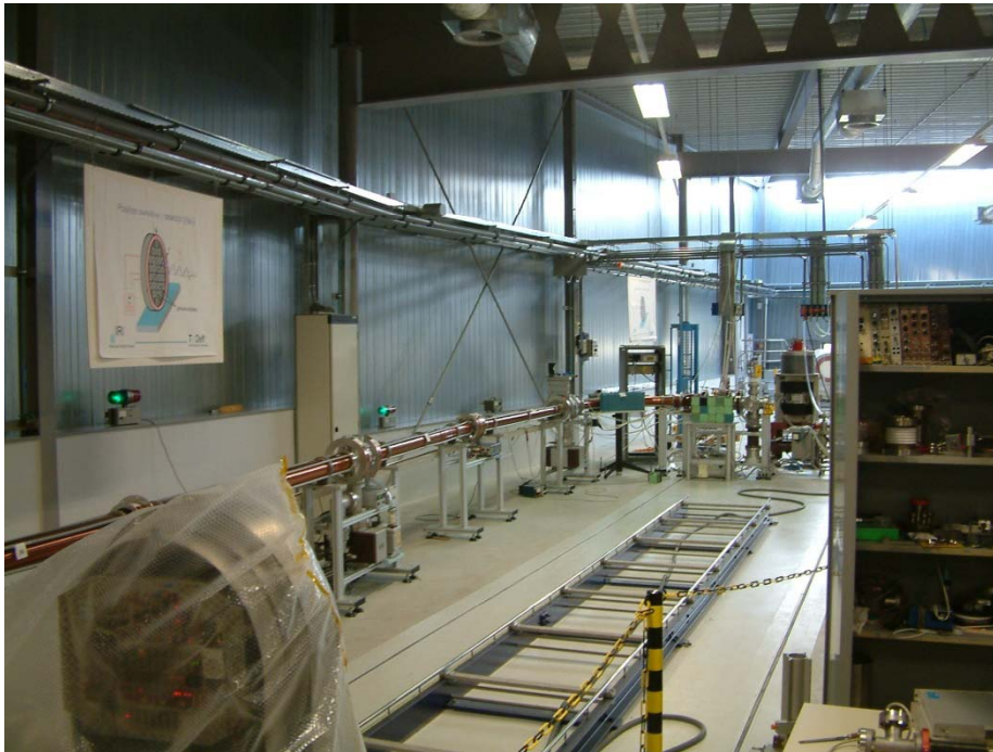
Beamline > 20 m, detector distance about 2x 10m
