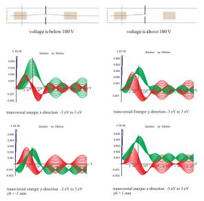
The green line shows the deflection in y direction , the black line the position of the chopper plates.
