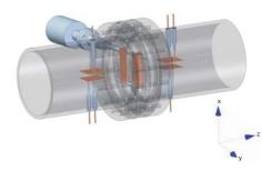
In z-direction, a magnetic field of 75 G is applied. If between two plates an electric field is applied in x-direction, the positrons obtain a transversal energy in that direction. Therefore, the radius of gyration is larger and the positrons can not pass the plates of the chopper. The pairs of plates with an antipodal electric field are spaced at intervals of one length of gyration (126 mm), so that the transversal energy is compensated when the positrons drop out of the chopper.
