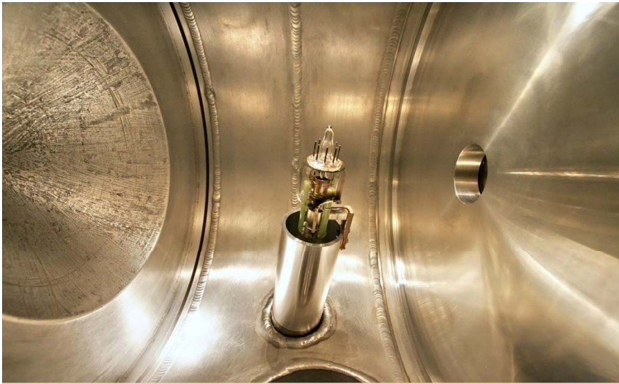
Test of Beam Guidance with an Electron Source
