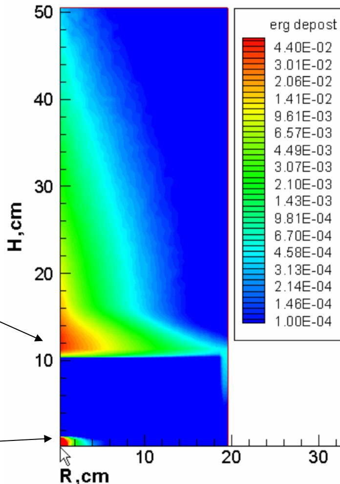
EPOS Density Energy Deposition (in MeV/cm<sup>3</sup>) for Distance = 10cm
