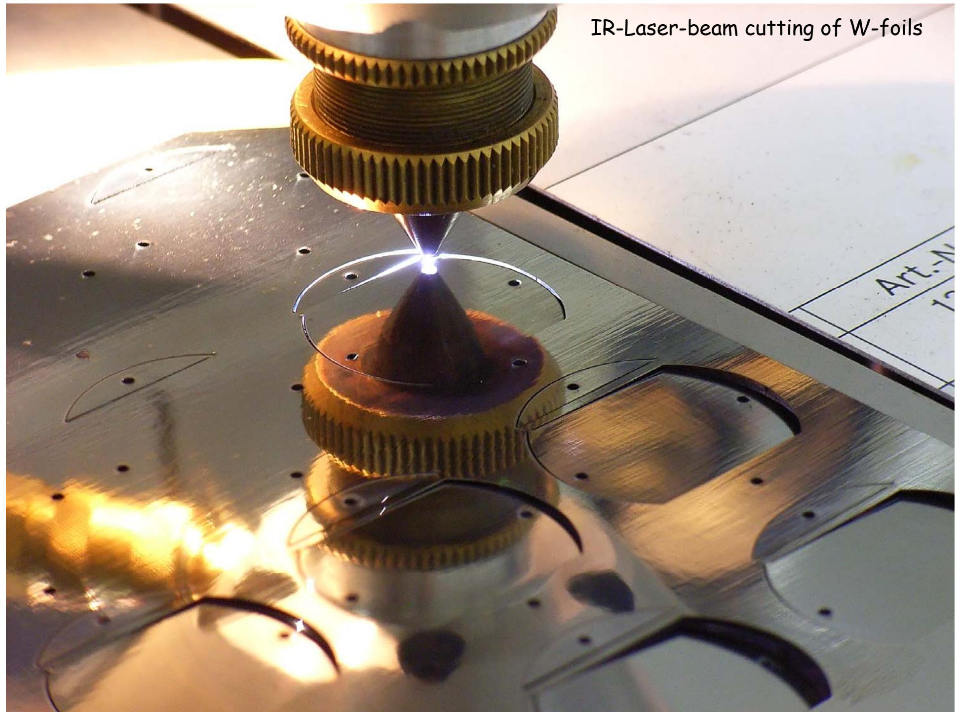
IR-Laser-beam cutting of W-foils
