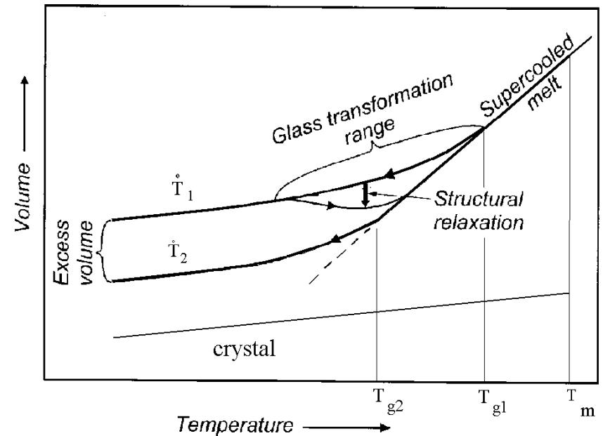
Glass transition  $T_g$  detectable via change in hole expansion
