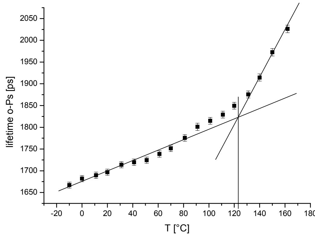
Increase in  $T_g$  (~ 120 °C) for intensively post-cured epoxy films
