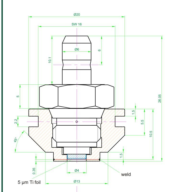
Each source capsule has been tested up to 5 bar overpressure. Moreover, the front part of each capsule was tested to be UHV tight down to 1E-8 Torr. The rear Al part contains a cavity for the neon gas which is created during the decay of 22-Na. A small hole at the side connects this cavity with the front part (see third photo).
