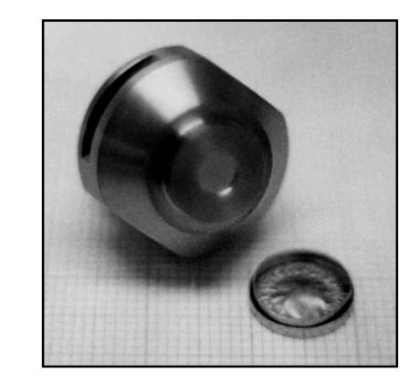
After closing the capsule (left photo), it is UHV tight (<10<sup>-8</sup> Torr). It can be reopened. The slits are made for the manipulator (see right column). In the positron beam system in Halle, the moderator sits directly on top of the source (right photo shows removed moderator). It is a W single crystal foil which is supported by a W ring.
