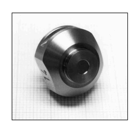
The rear part of the source capsule (left) is made from Al. The <sup>22</sup>Na isotope is evaporated on top of the Ta insert which acts as reflection plate. A small hole below the thread opens the volume behind the Ta piece for the created Ne gas. The right photo shows the front part which is completely made from Ti. A special design of the front ring ensures that the foil of the Ti window is drum-like spanned during welding.
