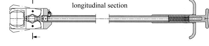
For easy manipulation, we constructed a pair of pliers. This allows a save handling without the necessity of touching the source (radiation protection). The source can easily be taken out of the transport container and can be mounted to the system. The complete set of drawings of the manipulator have been made at TU Munich and can be downloaded from our homepage as PDF version or as AutoCad files (www.ep3.uni-halle.de/positrons).
