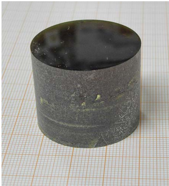
ZnO single crystal \varnothing 33 mm, grown at Inst. of Crystal Growth (IKZ), Berlin
