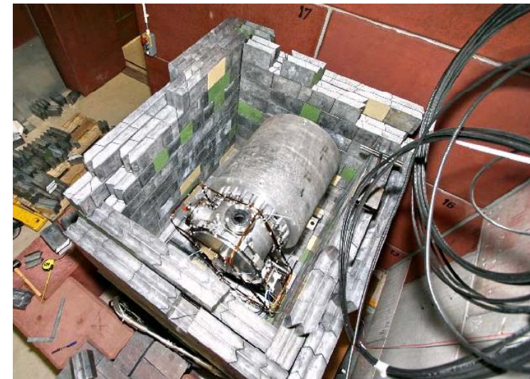
The electron to gamma to positron converter at EPOS (Rossendorf)
