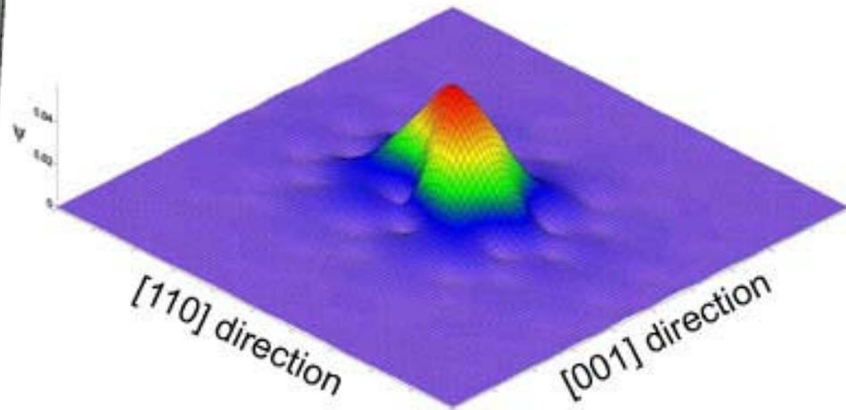
■ Vacancy represents a positron trap due to the missing nuclei (potential well for a positron)
