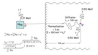
Positrons emerge in β+-radiation, for example in Ma<sup>22</sup>
