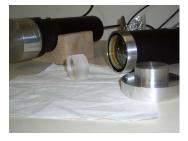
Scintillator Converts  $\gamma$ -ray into "visible" light of 220nm Photomultiplier Photons trigger (single) electrons, which are gathered, focused and multiplied. Result: a current and a voltage-peak
