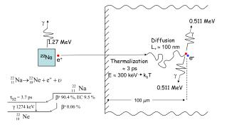
Positron annihilates with electron, 2 γ-quanta of 5<sup>44</sup> keV are emitted
